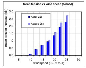
Fig. 4.5 Effect of wind only (no ice) on smooth (light blue) and stranded (dark blue) conductors of 19mm diameter
