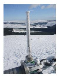
Fig. 5.1 The Combi-Tech ice monitor at Deadwater Fell
