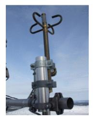
Fig. 5.3 The HoloOptic icemeter at Deadwater Fell
