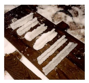
Fig. 2.5 Ice accretion samples from different conductors on test at Deadwater Fell.
