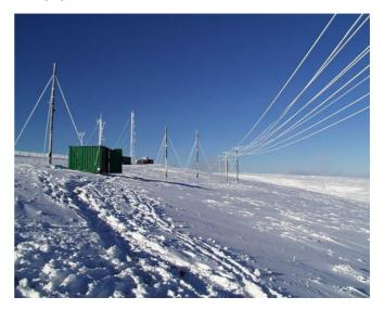
Fig. 2.2 The main test span and measurement huts plus poles for infra red lighting at the test site. In this picture intermediate single poles have been erected for testing small conductor sizes.
