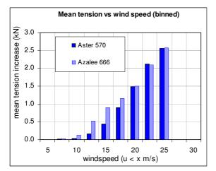
Fig. 4.5 Effect of wind only (no ice) on smooth (light blue) and stranded (dark blue) conductors of 31mm diameter
