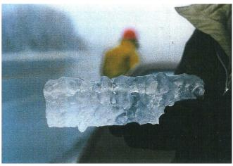
Fig. 2.6 Glaze icing sample from a conductor under test
