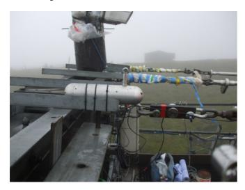
Fig. 3.2 Load cells and turnbuckles are installed on all conductors
